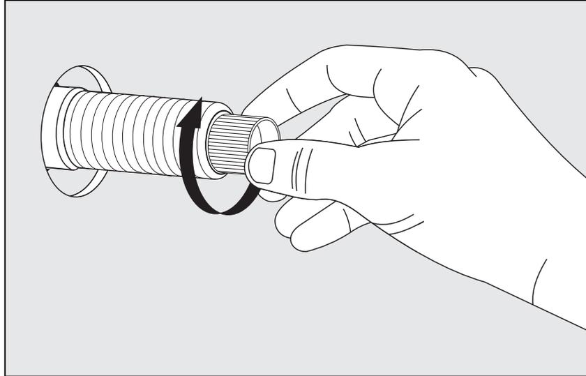
8- Place the handle by threading it's body on the brass extension.
