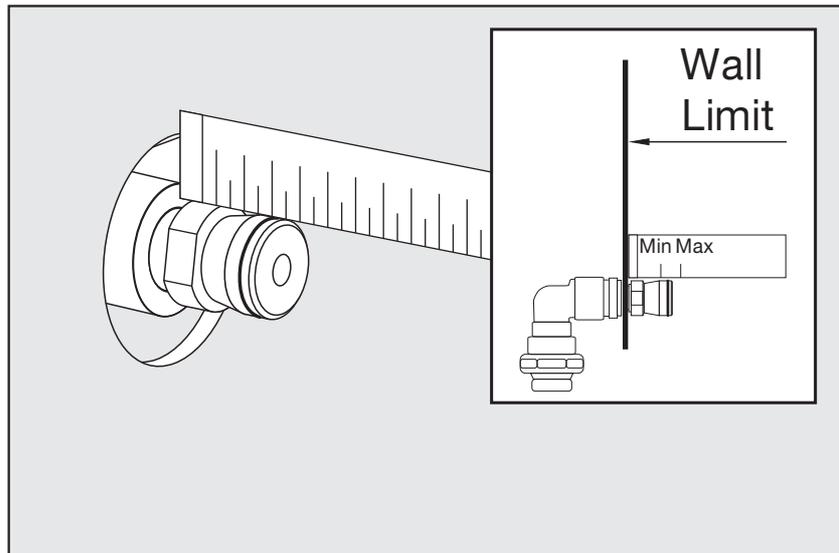
15 - To install the spout place it on the spout connector (is not necessary to thread it).
