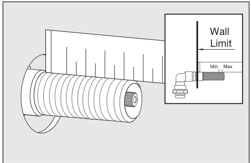
3 - **If the measured distance exceeds the "max" value** it's necessary to trim brass extension and valve stem (together).
