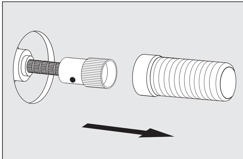
12- Remove, rotate, and reinstall the connector. And restart since point 6.
