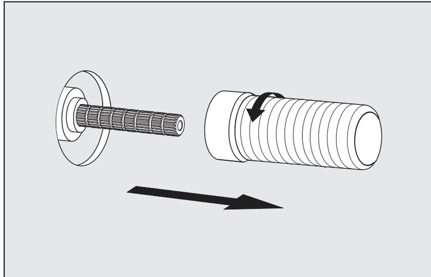
5- Place the connector and tight it with provided small allen wrench as shown in the picture.
