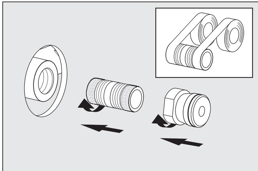
14 - Once placed the spout connector use a ruler to check the instalation distance against the wall.
