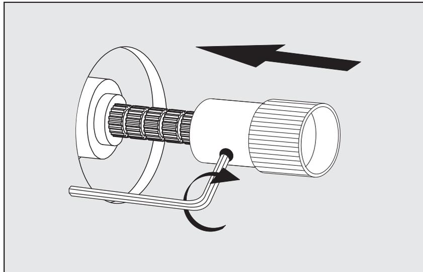
6 - After tightening the connector, place the brass extension.
